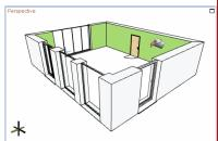
With the function "Dye Selection" you can assign the same color to groups of objects. This function is particularly useful when you draw floor-space plans since you do not have to dye each object individually. Select an arbitrary number of objects in your drawing. Click "Dye Selection" in the Materials group on the Edit tab and click one of the provided colors or define a color. The selected color will now be assigned to the selection of objects.
